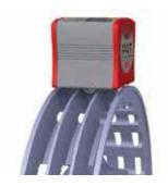
The Fixturlaser PAT units are very easily mounted on the pulleys. The spring action probe finds the center of the belt groove. The industrial built-in magnets snap the units to the pulley in a perfect fit.
